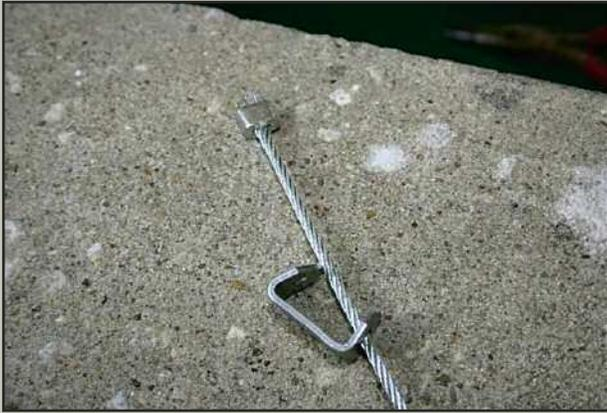
**Run the cable through the snare lock.**
