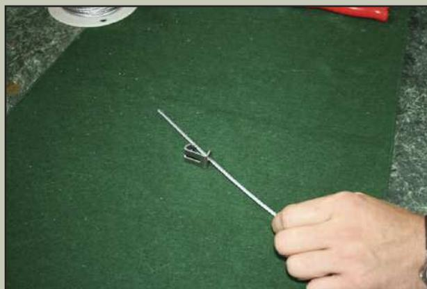
Run the cable through the snare lock.
