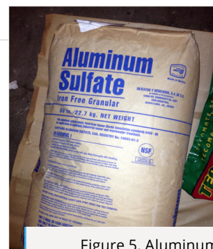
Figure 5. Aluminum sulfate, one of the “big guns” of clearing turbidity, is displayed in the image above. Due to its ability to rapidly lower the pH of pond water, it should only be used on ponds with an alkalinity higher than 50 ppm.
